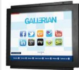
Chassis type Panel PC with flange for easy installation.
