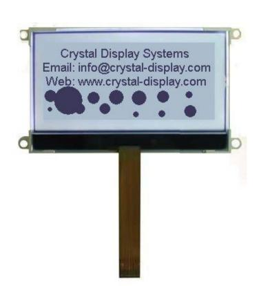
Our product line-up boasts a wide array of alphanumeric and graphic STN & FSTN LCD modules, incorporating cutting-edge COB/SMT and COG technologies.
