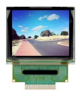
PMOLED technology outperforms traditional LCDs in small graphic displays. Many applications are shifting from monochrome LCD and TFT LCD to PMOLEDs for their superior visibility, fast response times, and low power consumption. PMOLEDs come in various sizes, offer full RGB colour, monochrome and area colour options, plus character displays compatible with standard LCD modules.
