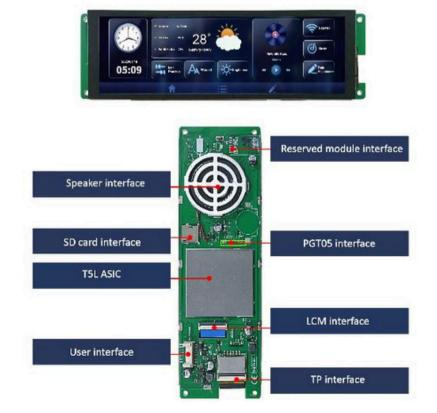
Designing a product with a colour TFT display and touch functionality is simplified with CDS's UART Display lineup, allowing rapid user interface (UI) development through an intuitive software tool. These displays utilize the **UART interface (TX & RX)** for seamless communication with microcontrollers and microprocessors, eliminating the need for complex display or touch drivers.
