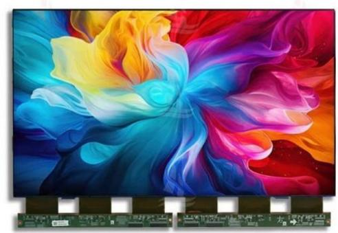
Our AMOLED display range stands at the forefront of high-performance display technology, offering unmatched optical specifications. Available in sizes from 0.95" (120RGBx240) to 27.0" (4K), these displays are engineered for applications that demand superior quality and responsiveness.
