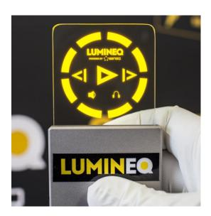
The ELT15S-1500 is a high brightness TASEL® transparent segmented display demonstrator that exhibits the full see-through properties of a TASEL display, be that for functional or aesthetic reasons.
