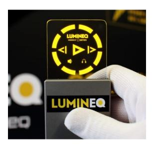
The ELT15S is a TASEL® transparent segmented display demonstrator that exhibits the full seethrough properties of a TASEL display, be that for functional or aesthetic reasons.
