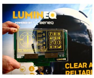
The ELT256.120.90 is a TASEL® transparent matrix display designed for use in applications requiring full see-through properties of the display, be that for functional or aesthetic reasons.
